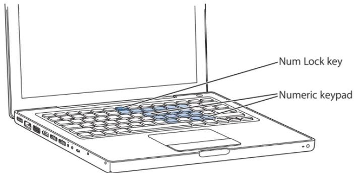
To use the numeric keypad, press the Num Lock key. An indicator light on the Num Lock key glows when the keypad is active. When you finish using the keypad, press the Num Lock key again to turn it off.
