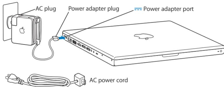
To extend the reach of your power adapter, you can attach the AC power cord. First pull up on the AC plug to remove it from the adapter, and then attach the included AC power cord to the adapter. Plug the other end into a power outlet. For an illustration, see page 31.
