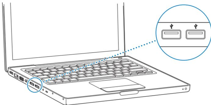
To use a USB device with your computer, connect the device to the computer. Your computer automatically detects newly connected devices and loads the correct software to work with the device.
