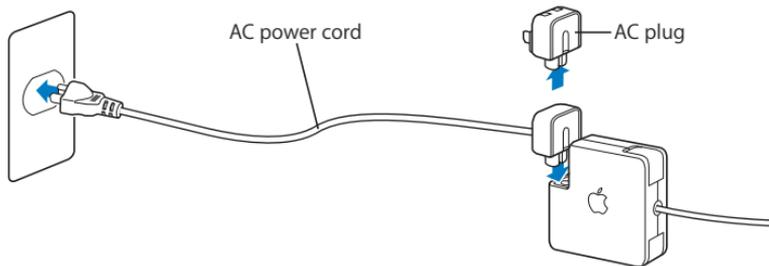
Use the AC power cord and connect it to a grounded power outlet when one is available. Use only the AC power cord that came with your power adapter. Make sure to push the power plug snugly into the power adapter port on the computer to ensure it is engaged and power is flowing to the computer. If the cord is plugged in properly, you'll see a glowing indicator light on the end of the cord that plugs into your MacBook.
