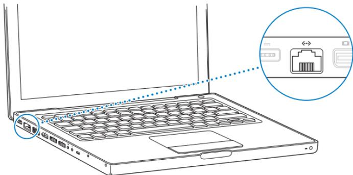
Connecting to a network gives you access to other computers and potentially to network printers, modems, email, and the Internet. You can use Ethernet to share files between two computers or set up a small network. The Ethernet port on your MacBook automatically detects other Ethernet devices. You don't need an Ethernet crossover cable when connecting to other Ethernet devices.
